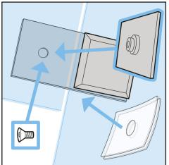
4. Next install the door aperture glass Next, install the upper glazing of the door aperture. First attach the glass brackets to the side glass (or to the wall if there is no side glass) When fixing to the wall, first check the position of the fixing hole in the glass on the other side of the side glass.
