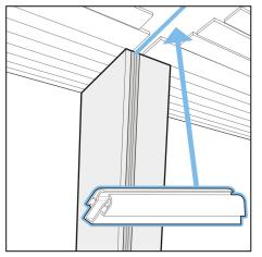
1. Drill holes in the bottom of the top moulding (flush moulding) for the fixing screws where it is to be fixed to the vapour barrier timbers, or at a pitch of about 600mm if the vapour barrier timber is integrated.
