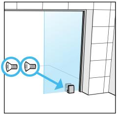
3. Once the mouldings and the floor bracket are installed, place the glass on the mouldings and the floor bracket. Tighten the rear part of the floor bracket with screws.
